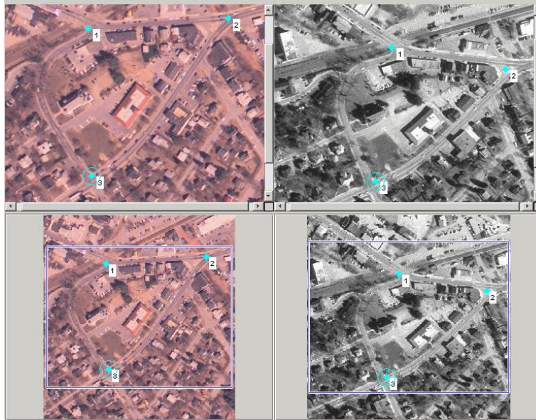
Fig.2. (a) Reference Image, (b) Reference Image Feature points, (c) Sensed Image, (d) Sensed Image Feature points
