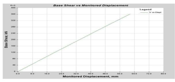
Fig 3.6 Push-Over curve of the Ferro cement infilled frame G+3 building model 5
