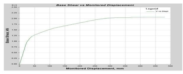
Fig 3.1 Push-Over curve of the model 3 bare frame G+3 building
