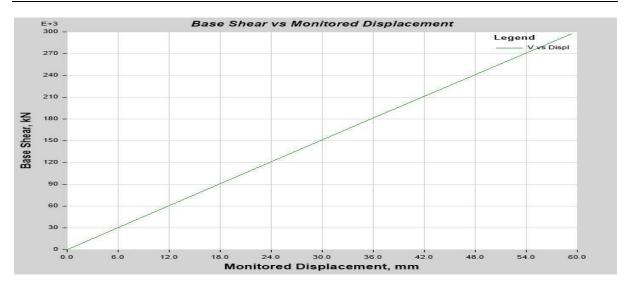
Fig 3.8 push-Over curve of the Ferro cement infilled frame G+9 building model 5
