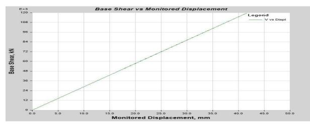
Fig 3.4 Push-Over curve of the brick infilled frame G+9 building model 3
