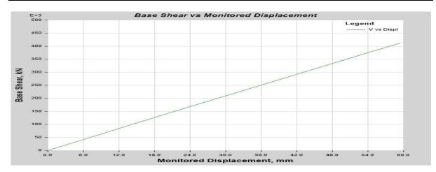
Fig 3.5 Push-Over curve of the Ferro cement infilled frame G+3 building model 3
