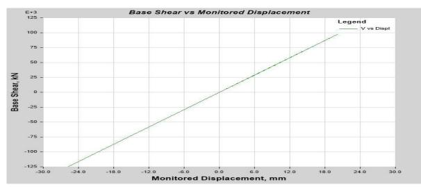
Fig 3.7 Push-Over curve of the vertical Ferro cement frame G+9 building model 3
