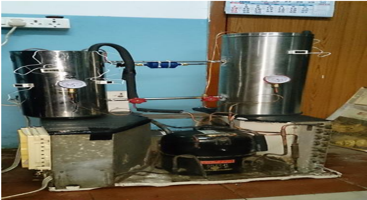
Fig 1.4: Air conditioning cum Water Dispenser System
