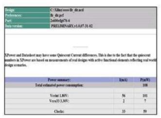
Fig.8. Power Analysis of FIR filter using proposed design.
