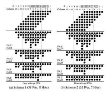
Fig. 2. Tree reduction of 8 × 8 multiplication Scheme 1 and (b) Scheme 2 in Table I. (a)
