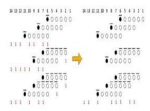
Fig.3. Generation of PPBs considering sign extension and negation.
