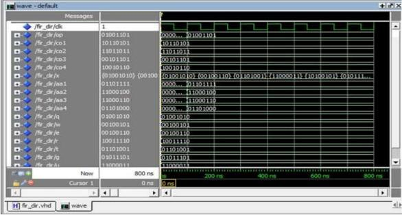
Fig.7. Simulated result of FIR filter using proposed design
