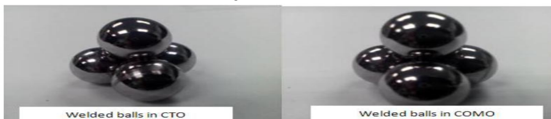
Fig 4.7 Welded balls in the experimental oil
