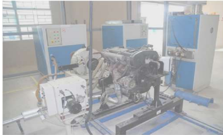
Figure 1: Mitsubishi 4D68 SOHC 2.0 L Diesel Engine Testing rig
