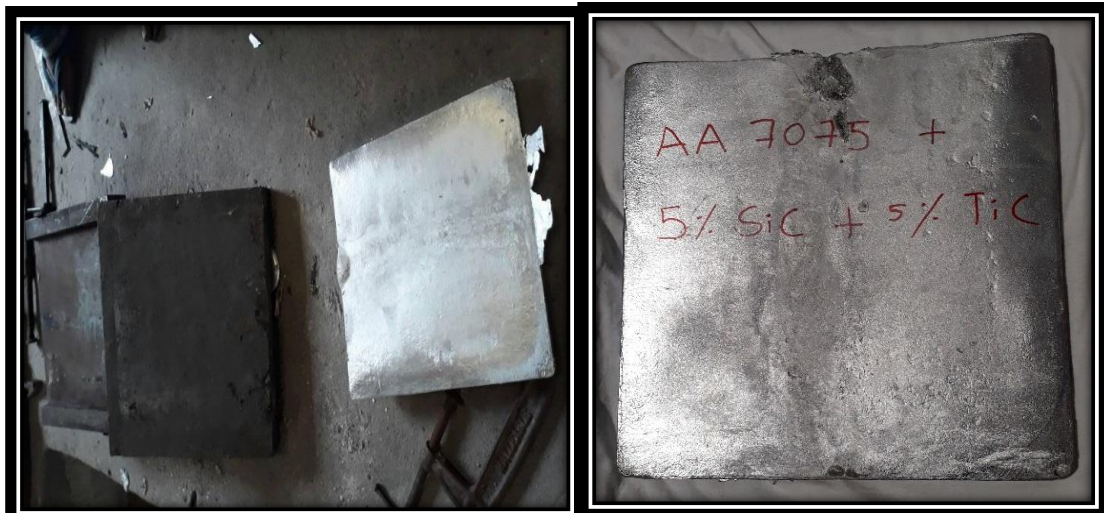
Fig. 3 HMMC of AA7075 with 5% SiC and 5% TiC
