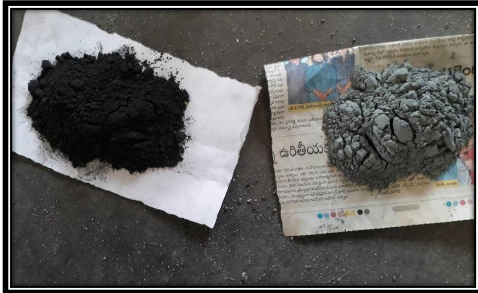
Fig. 2 SiC powder and TiC powders added to molten AA7075
