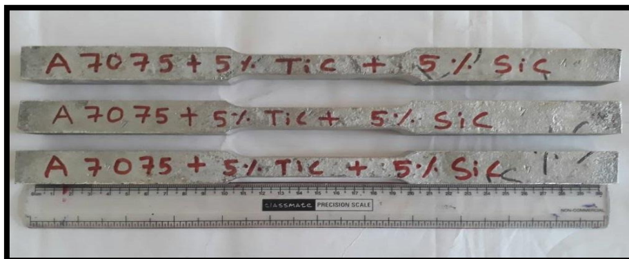
Fig. 5 Tensile Specimens of AA7075-SiC and TiC composites before fracture
