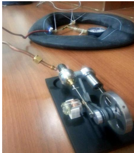
Fig.2. Electricity Generation with StirlingMotor
