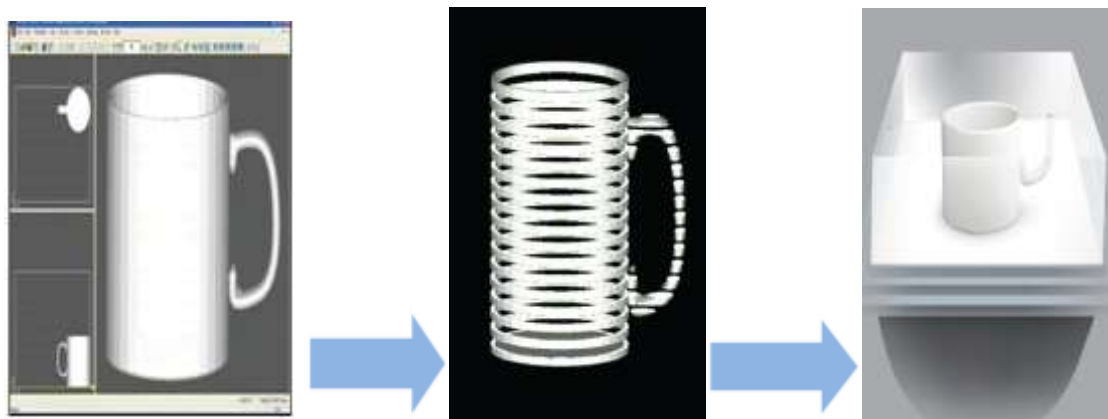
Fig:2 Layered Manufacturing: Concept-Model-Slicing-3D Printing
