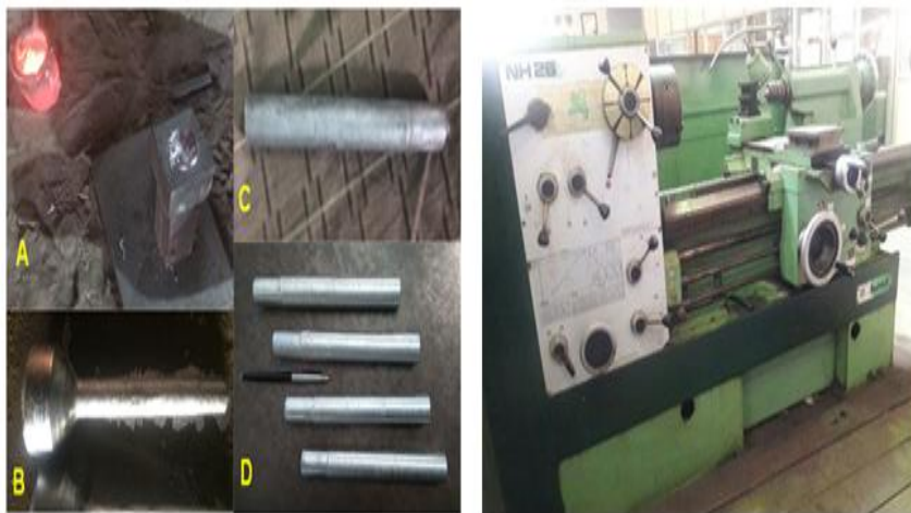
Fig. 1 – A: Casting Process, B: Casting, C: Experimental Setup: Finished Workpiece, D: Workpiece After Machining
