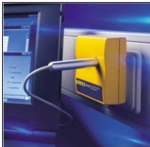
Fig.8. Event data link by optical interface cable between computer and VR101
