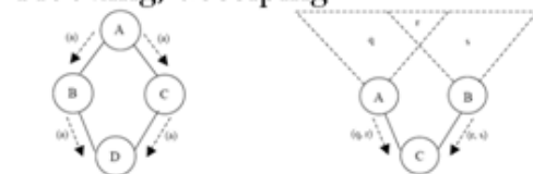
Fig. 1: The implosion problem. Node A starts by flooding its data to all of its neighbors. D gets two exact copies of data eventually, which is not necessary. Fig. 2: The overlap problem. Two sensors cover an overlapping geographic region and C gets some copy of data from these sensors.
