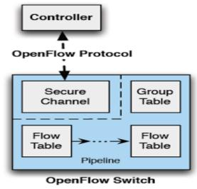
Fig. 5 Open Flow Switch
