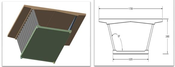
Fig.2 Ansys And Autocadd Model Of Trapezoidal Composite Box Girder
