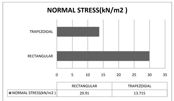
Fig.5 Graph Showing Normal Stress Of Two Models
