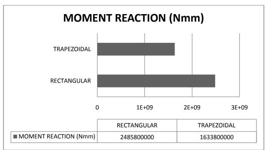
Fig.7 Graph Showing Moment Reaction Of Two Models
