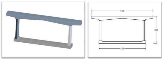
Fig.1 Ansys And Autocadd Model Of Rectangular Composite Box Girder
