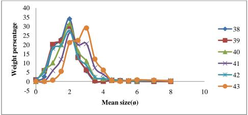
Fig.13. Frequency Distribution Curves of Surface Sediments of Lower Estuary Bar(4) of Gosthani River.
