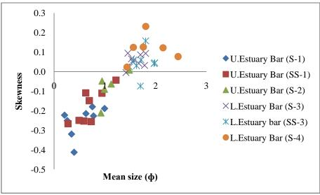
Fig.3.Scatter Plot between Mean Size Vs. Skewness of Estuary Bar Sediments.
