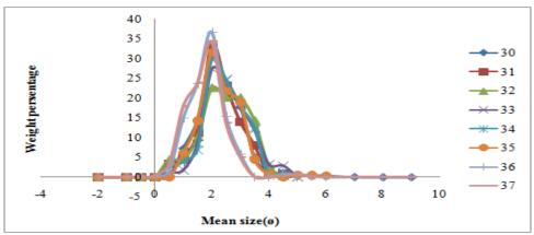
Fig.12.Frequency Distribution Curves of Sub-Surface Sediments of Lower Estuary Bar(3) of Gosthani River.
