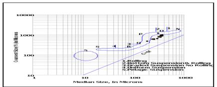
Fig.15.Complete CM Pattern of Tractive Current Deposits of Estuary Bar Silt and Clayey Sediments
