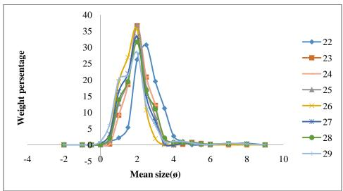
Fig.11. Frequency Distribution Curves of Surface Sediments of Lower Estuary Bar(3) of Gosthani River.
