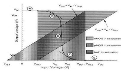
Fig 2: Operating region of n-MOS and p-MOS transistor [1]
