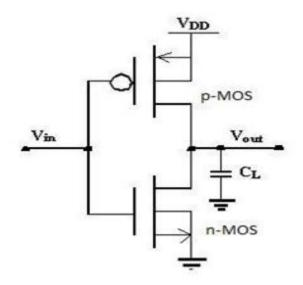
Fig 1: Structure of CMOS inverter
