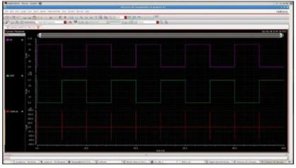
Fig 5: Transient behavior of CMOS inverter (i) VIN (ii)VOUT (iii) IC
