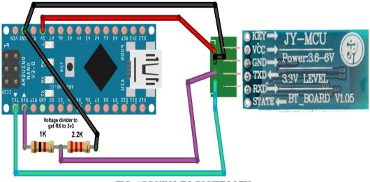
FIG. ARDUINO TO BLUETOOTH
