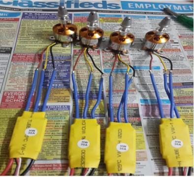
FIG. BRUSHLESS MOTOR AND ESC
