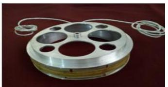
c. Coil former Fig. 3 Different parts of newly fabricated compressor
