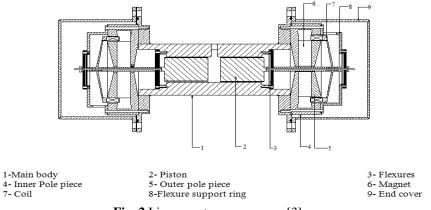
Fig. 2 Linear motor compressor [3]
