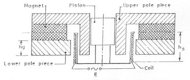
Fig. 1 Moving coil linear motor [3]
