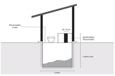
Figure 2. Scheme of a dry toilet.
