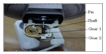
Fig. 2: Oscillating Mechanism of Standing Fan
