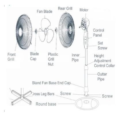
Fig. 1: Assembly of Standing Fan
