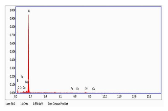
Figure 3a:EDS spectrum of Al-2024 alloy
