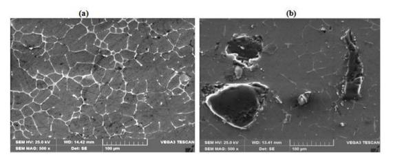
Figure 2. a-b Showing the scanning electron microphotographs of (a) as cast Al2024 alloy (b) with 4 wt.% of  $B_4C$ .
