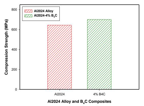
**Figure 5:** Compression strength of Al2024 and 4 wt. % of micro  $B_4C$  composites The plot 5 indicates the compression strength of the test specimens with 4 wt.% of  $B_4C$  in Al2024 alloy. Here 12% increase in the compression strength indicates that there is an opposition for the moment of dislocations along the boundary of the composite.
