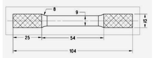
Figure 1: Tensile specimen according to ASTM E8 with all dimensions in mm
