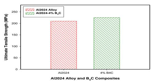
Figure 4a: Ultimate tensile strength of Al2024 and 4 wt. % of micro B<sub>4</sub>C composites
