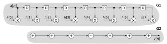
Fig 3.1 (B) Decomposition Of Dfg To Two Subgraphs G1 And G2 For Feed-Forward Cutset Retiming Of Dfg.
