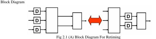
Retiming Means Changing The Position Of Existing Delay Elements. Retiming Improves Circuit Performance By Optimizing Combinational Delay. Difference Between Retiming And Pipelining Is Retiming Does Not Change The Input/Output Behavior Of The System.
