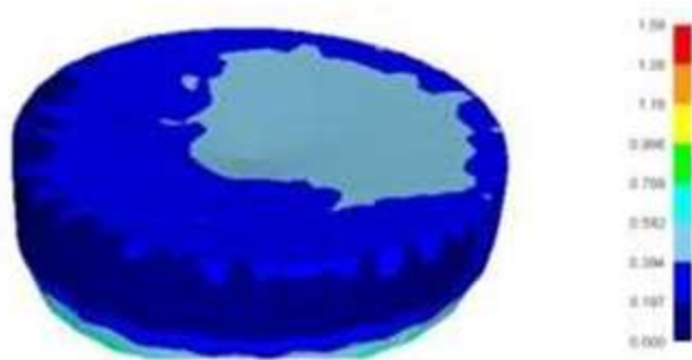
Figure 2.5: Contour Plot of Effective Strain (mm/mm) during rotary Forging.
