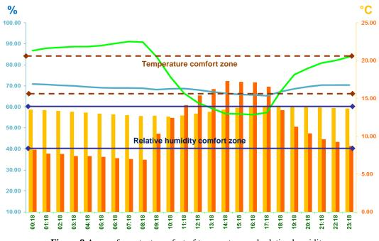
Figure 9. Areas of constant comfort of temperature and relative humidity Typical day of residential housing in January
