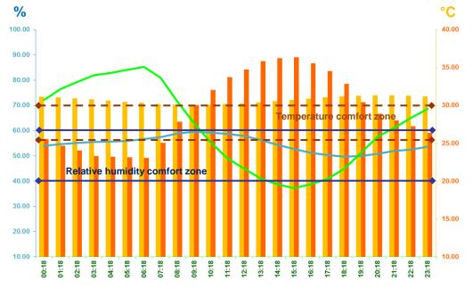
Figure 11. Areas of constant comfort of temperature and relative humidity Typical day of residential housing inAugust
