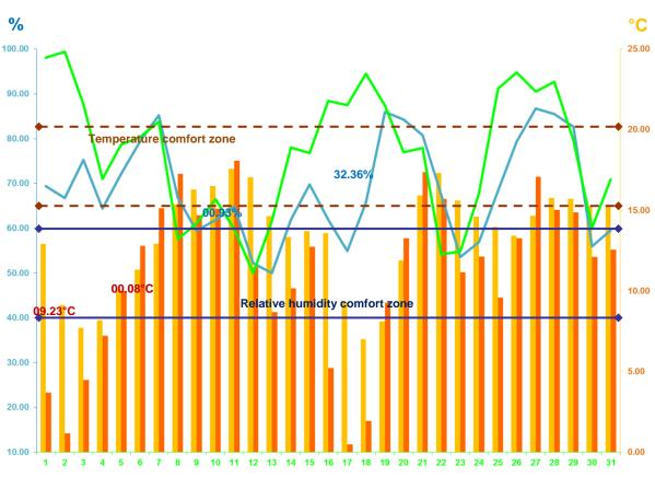
Figure 8. Areas of constant comfort of temperature and relative humidity in January
