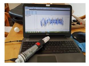
Figure 7. Obtaining data from Hobo Pr0 V2 U23-001
