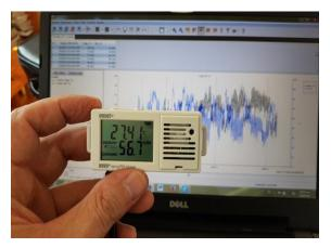
Figure 6. Obtaining data from Hobo UX100-003
