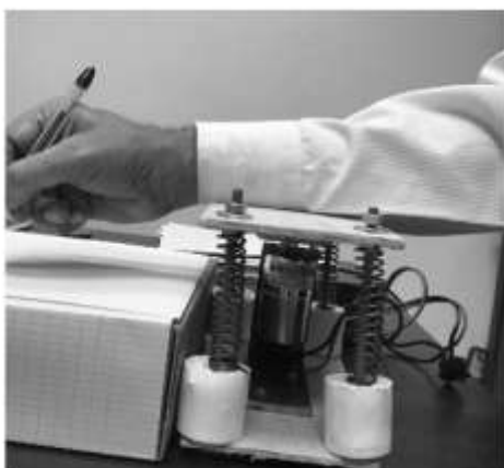
Fig. 2. Spiral drawing data acquisition from the tremor simulator.
