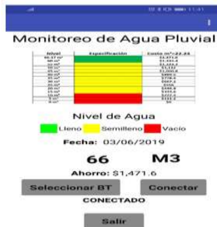
Figure 8. Interface that shows the cubic meters and the savings generated with the Rainwater Collection System.
