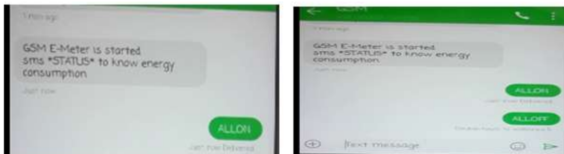
Fig.1.4 SMS FROM MOBILE FOR SWITCHING ON/OFF THE APPLIANCES
