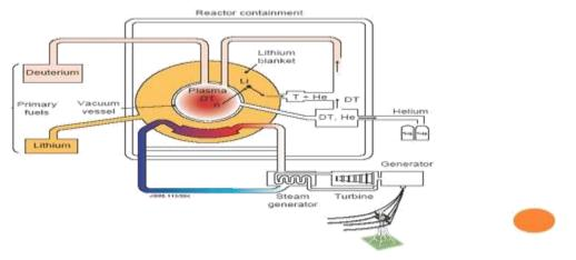
Fig 1. Working of ITER
