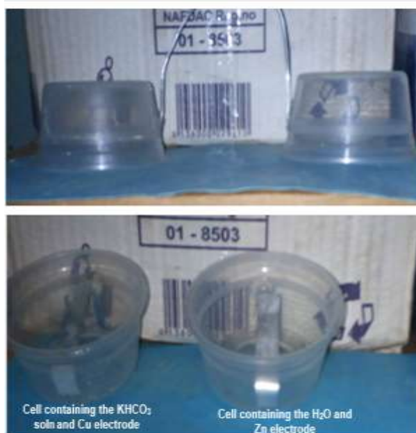
Figure 2: View of the half-cell compartments with Zinc and Copper electrodes
