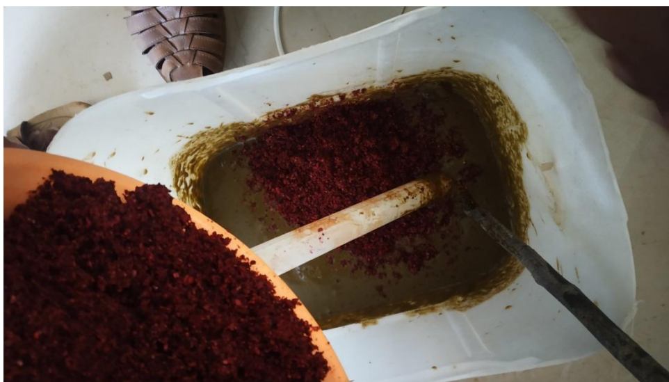
Fig.5: Mixing powdered waste with sludge
