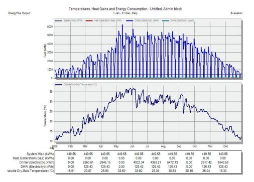
Figure 6 Monthly Report of HVAC Energy Consumption (Design Builder Software)
