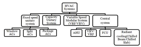
Figure 7 Various Types of HVAC Systems Discussed in Analysis (source: NBC 2016)
