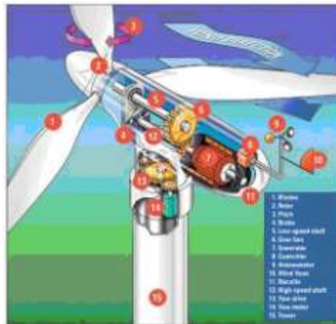
Fig. 1. Horizontal axis wind Turbine
