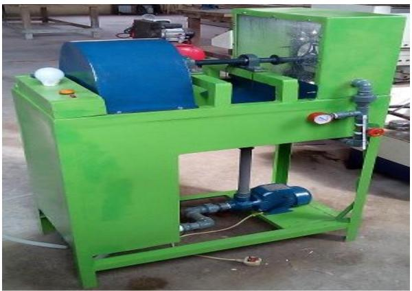
Figure 3.4: The Manufactured Pelton wheel (Impulse Turbine) in AkwaIbom State University's Workshop
