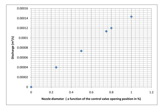
Figure 4.2: Shows the effect of Nozzle diameter on the Discharge of the turbine
