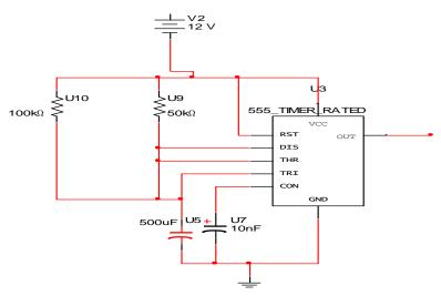
Figure. 5 The schematic diagram of the Astable 555 timer
