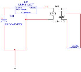
Fig. 4 Diagram of the cut-off switch
