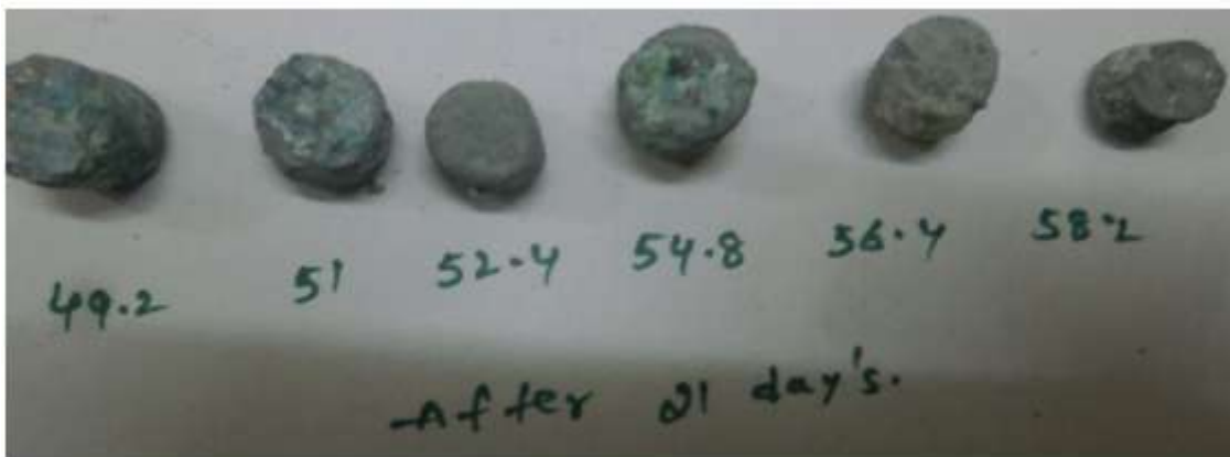
Fig4.4B. Corrosion Test Samples after 21 Days
