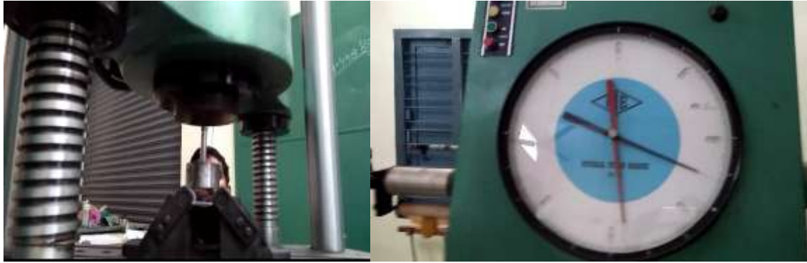
Fig 3. Shows applying a load 40KN by using UTM
