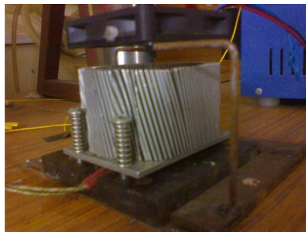
Figure 2. Copper heater block and aluminium sink used in the experimental set up
