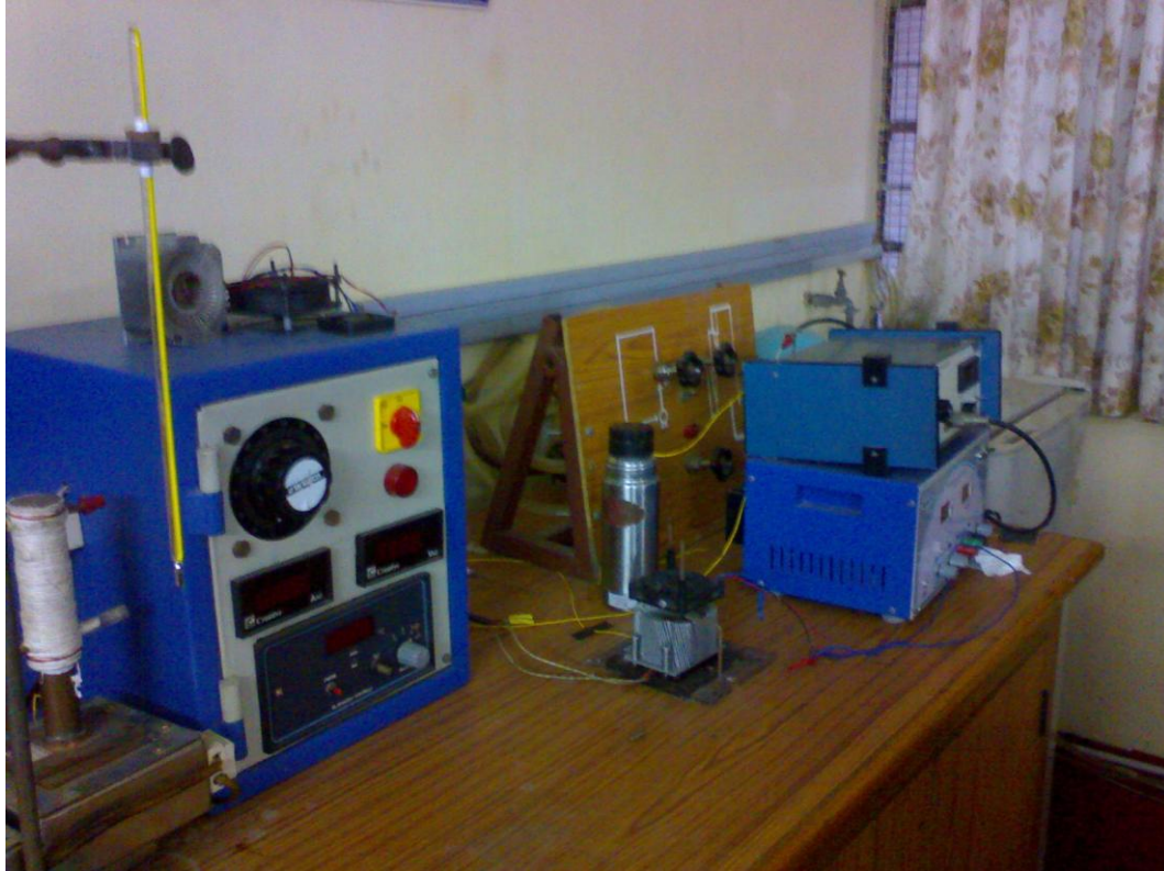
Figure 4. Experimental set up for finding thermal contact resistance of TIM
