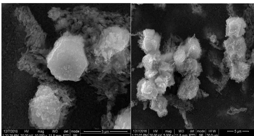
**Fig.2(c)** SEM image of TiO<sub>2</sub>- ZnO film **Fig.2 (d)** SEM image of TiO<sub>2</sub>- ZnO film
