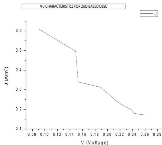
**Fig.4(b)** J-V characteristics of ZnO
