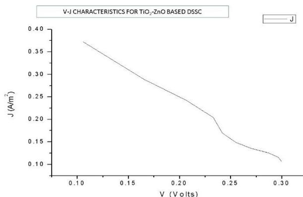
**Fig.4(c)** J-V characteristics of TiO<sub>2</sub>-ZnO
