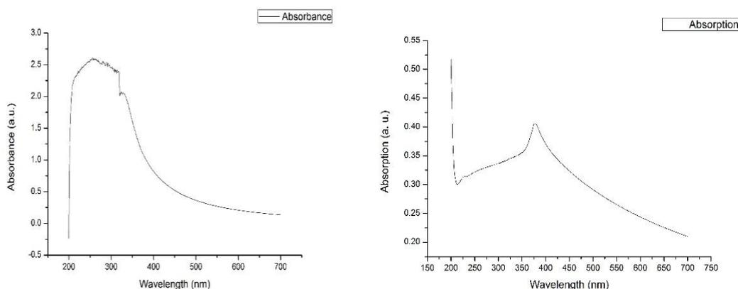
**Fig.3 (a)** UV-Vis Absorption for TiO<sub>2</sub> **Fig.3 (b)** UV-Vis Absorption for ZnO
