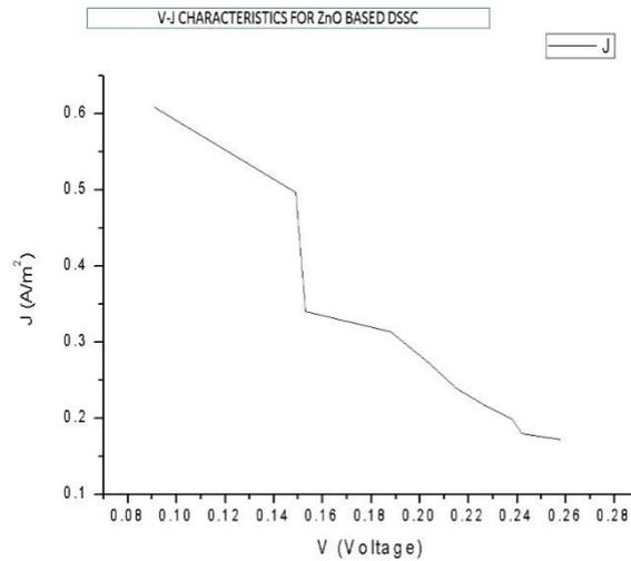
**Fig.4(b)** J-V characteristics of ZnO
