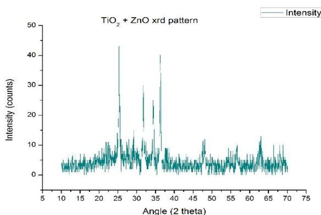
**Fig.1(c)** XRD image of TiO<sub>2</sub>- ZnO films.
