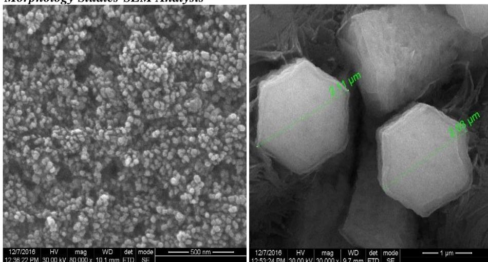
**Fig.2(a)** SEM image of TiO<sub>2</sub> **Fig.2(b)** SEM image of ZnO
