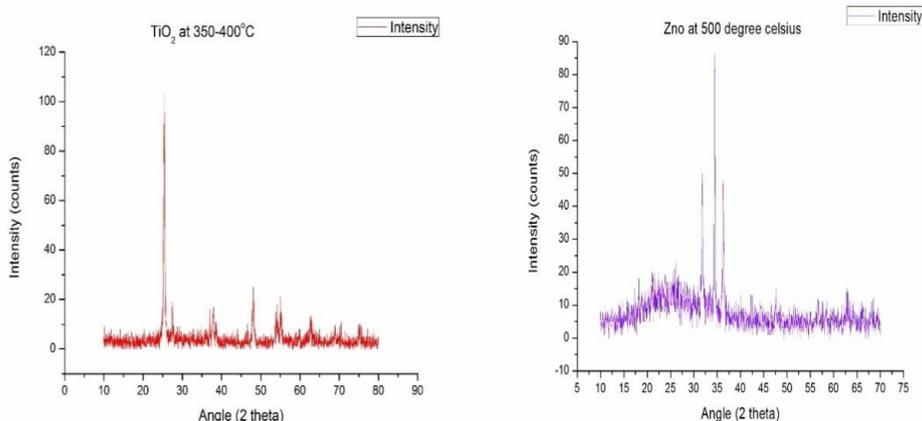
**Fig.1 (a)** XRD of TiO<sub>2</sub> coating annealed at 350°C **Fig.1 (b)** XRD of ZnO coating annealed at 500°C
