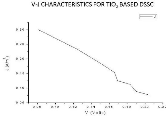
**Fig. 4(a)** J-V characteristics of TiO<sub>2</sub>
