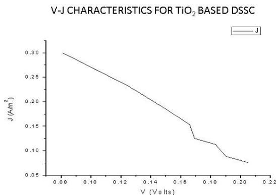
**Fig. 4(a)** J-V characteristics of TiO<sub>2</sub>
