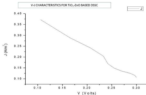
**Fig.4(c)** J-V characteristics of TiO<sub>2</sub>-ZnO
