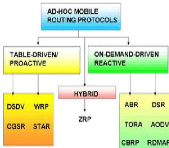
Fig 4-Ad-hoc Mobile Routing Protocols
