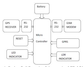
Fig.3 Automatic Broken Rail Detection Scheme using LED-LDR Assembly
