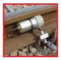
Fig.1 Ultrasonic Broken Rail Detector
