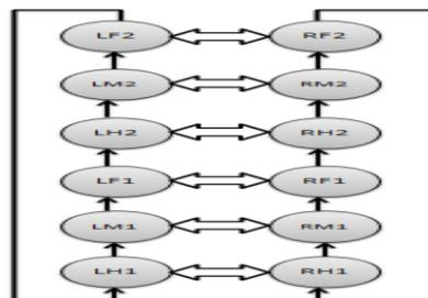
**Fig.2:**CPG locomotor model for hexapods, hexapod-robot. LF (left fore leg), LM (left middle leg), LH (left hind leg), RF (right fore leg), RM (right middle leg), RH (right hind leg).
