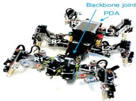
**Fig.3:AMOSII, each degree of freedom is controlled by an oscillator and the inter limb coordination is provided by the connections between oscillators.**
