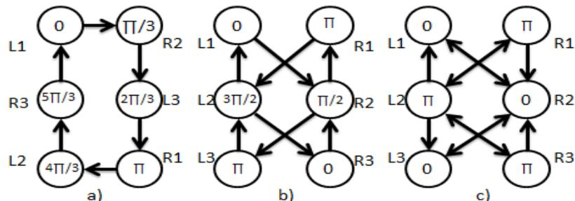
**Fig.4: Configuration of typical gait patterns in hexapod locomotion and the relative phases between limbs. The gaits are: (a) slow walk (b)Medium walk (c)fast walk.**
