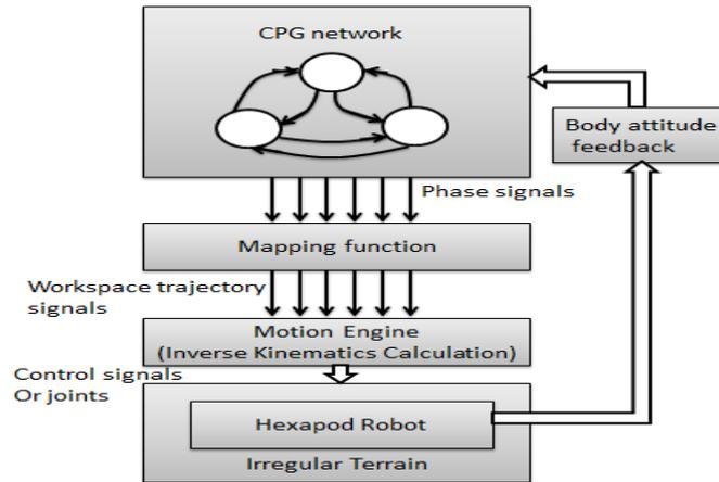
**Fig.6: Architecture of the locomotion control system**
