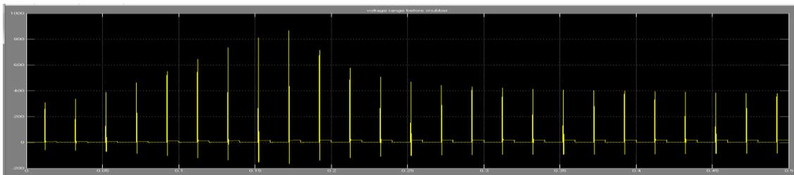
Fig7: Voltage Range Before Snubbers
