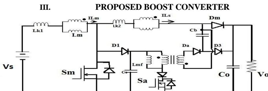
Fig.2: boost converter with snubber and ZVS
