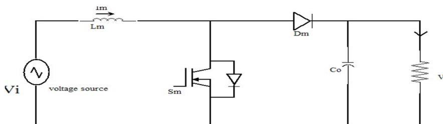
Fig.1: Normal boost converter
