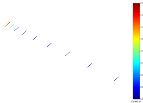
Figure 13. Current Distribution at 2.3GHz
