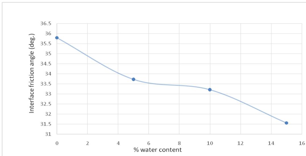
Figure 7: Variation of interface friction angle between tested soil & woven geotextile with water content
