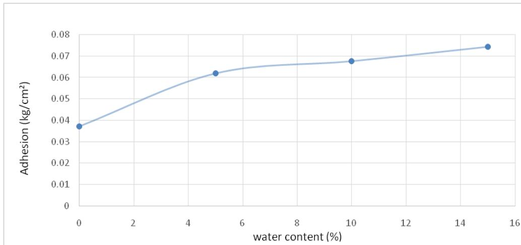
Figure 6: Variation of adhesion between tested soil & woven geotextile with water content
