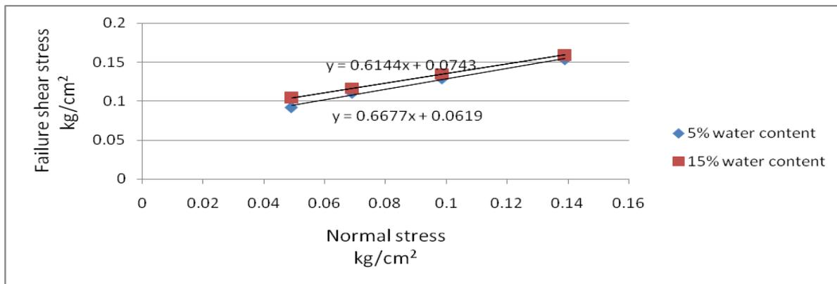
Figure 5: Sliding shear test results (Soil sample with 5% & 15% water content)
