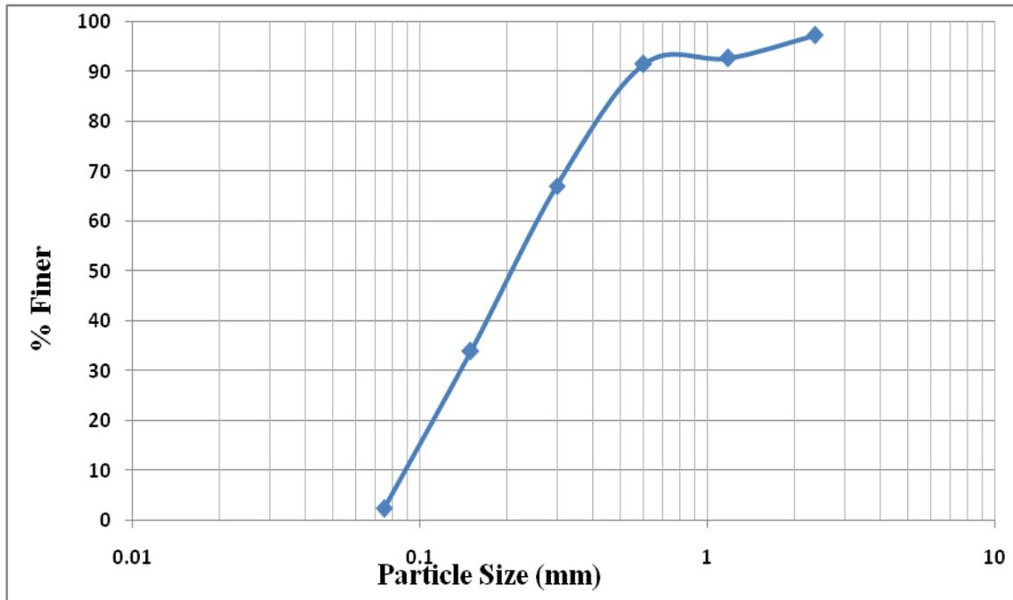
**Figure 3: Particle size distribution curve of experimental soil**
