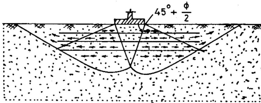
Figure 2: Sliding resistance (dense sand) [3]
