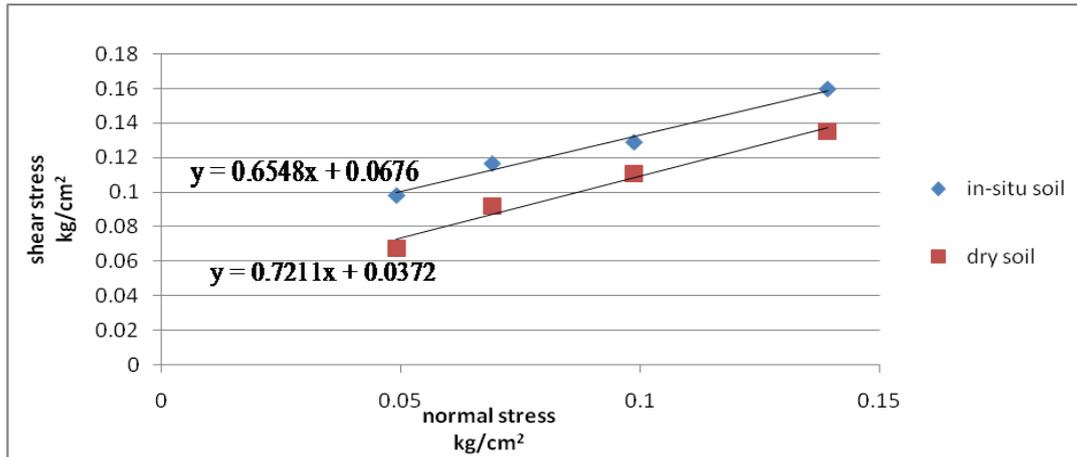
Figure 4: Sliding shear test results (In-situ & dry soil sample)
