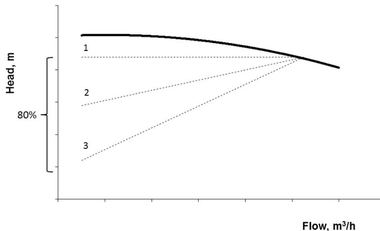
**Figure 1 Pumps' control modes (1 – constant pressure; 2-3 – proportional pressure with linear influence)**
