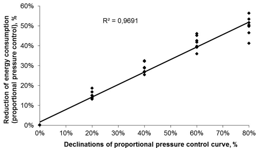
**Figure 3 Reduction of energy consumption applying proportional pressure control (vs. constant pressure)**
