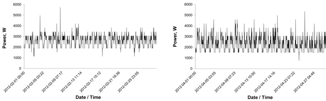
Figure 8 Power values (from left: constant pressure; from right: proportional pressure)
