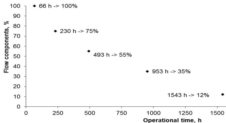
Figure 5 Load profile of network pumps in public water supply system
