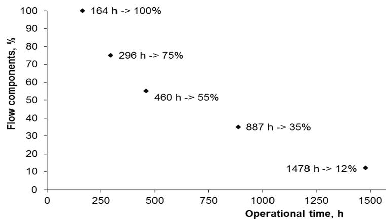
**Figure 2 Theoretical load profile of network pumps in public water supply**
