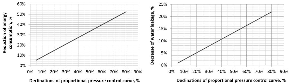
**Figure 11 Interaction among energy consumption, water leakage, and declination of pump proportional pressure control curve**
