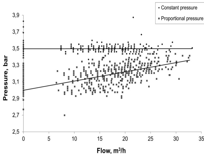
Figure 10 Pressure and flow values applying constant and proportional pressure control
