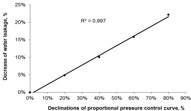
**Figure 4 Annual decrease of water leakage from current water leakage rate applying proportional pressure control (vs. constant pressure)**
