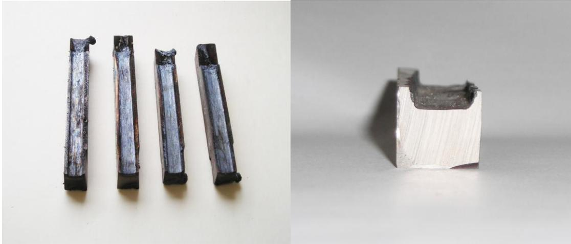
Figure 2. Four HSS test pieces 12mm wide.
