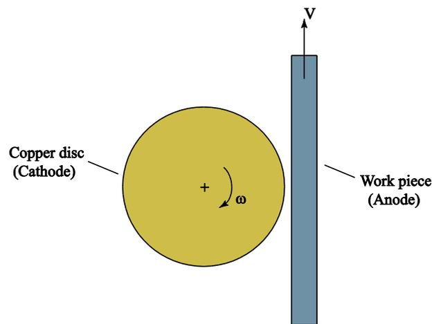
Fig. 2 Schematic sketch of the arc ablation process for developing a process model
