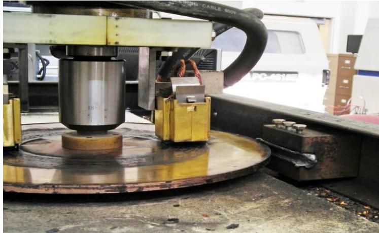
Figure 1. Experimental set-up with copper disk and high speed steel workpiece.
