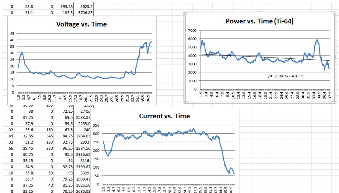
Figure 3. Electrical Measurements during a Ti-64 Grooving Experiment.
