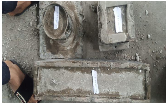
Fig 1: Cement slurry cured in mould
