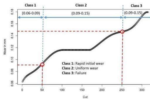
**Figure 2.** Flank wear progression according to the number of cut, and the wear classes.
