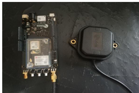
Figure 3 A u-blox CO99-F9P with ZED-F9P Global Navigation Satellite System receiver attached to its satellite.
