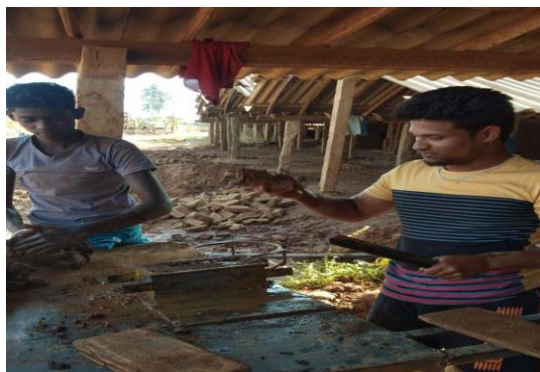
Fig. 5. Casting on Bricks
