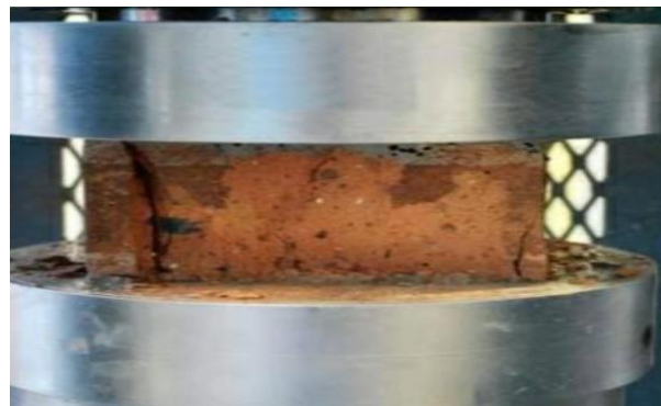
Fig. 5. Testing of Bricks
