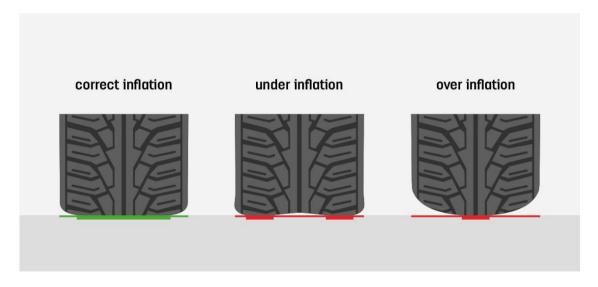
In the case of inflation, the tire profile, which is consistent with the above-mentioned data, reveals less tire contact with the earth, resulting in reduced road grip and braking force.
