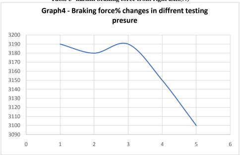
Graph 4 shows the relation between changing the inside pressure with changing of braking force is an exponential function. While inflation of tire has a negligible effect on decreasing braking force.
